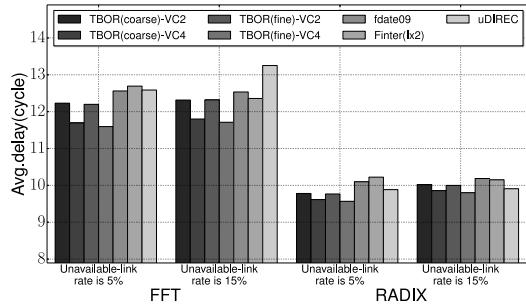
Fig. 8. Latency graphs for the FFT and RADIX SPLASH-2 benchmarks.
