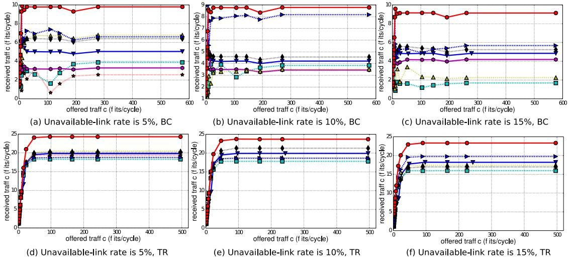
Fig. 6. —●— TBOR(fine)-VC4, —●— TBOR(fine)-VC2, —◆— TBOR(coarse)-VC4, —▲— TBOR(coarse)-VC2, —■— Finter(Ix2)-VC4, —★— Finter(I)-VC4, —○—  $f_{DATE09}$ -VC4. —▼— uDIREC-VC4. Load-throughput graphs for benchmarks on  $8 \times 8$  2D mesh with two or four virtual channels. We ran the same experiment on other traffic patterns (SHUFFLE and H.264), the results exhibited the same feature and we omit them here for brevity.<sup>2</sup>
