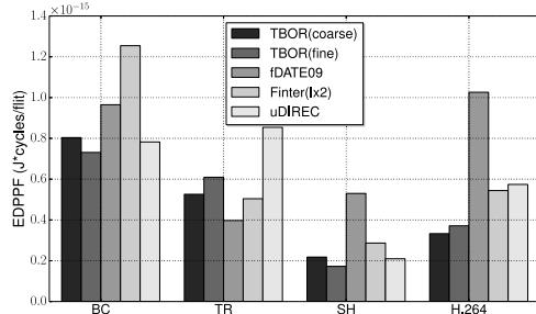
Fig. 10. Energy-delay product per flit derived from HORNET and DSENT, faulty or unavailable links rate is 10 percent. 10,000,000 flits were sent and delivered in each case.
