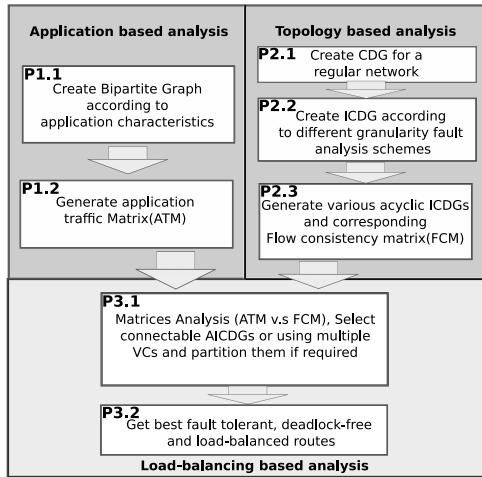
Fig. 2. Flow of the TBOR routing algorithm: the generated channel dependency graph of the irregular network (ICDG) is different for the fine- and coarse-grained techniques.
