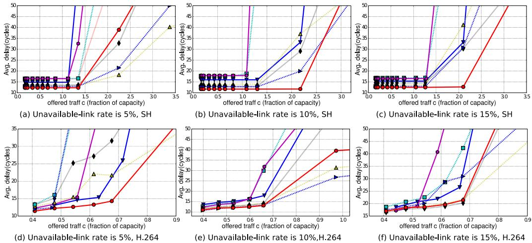
Fig. 7. —●— TBOR(fine)-VC4, —→— TBOR(fine)-VC2, —◆— TBOR(coarse)-VC4, —▲— TBOR(coarse)-VC2, —■— Finter(Ix2)-VC4, —○— fDATE09-VC4, —▼— uDIREC-VC4. Latency graphs for benchmarks on  $8 \times 8$  2D mesh with two or four virtual channels.<sup>3</sup>
