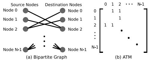
Fig. 3. Application traffic matrix derived from Bipartite graph, represent all the communication behavior of application.
