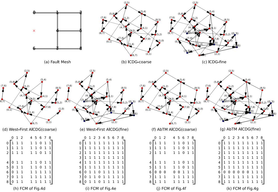
Fig. 4. CDGs for a  $3 \times 3$  2D mesh without virtual channel.
