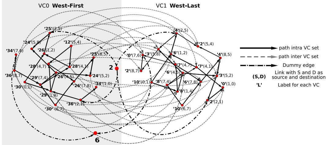
Fig. 5. An AICDG constructed with two VC sets: VC0 and VC1 apply West-First and West-Last respectively. VC0 is assigned a higher priority than V1. The VC labels are in bold type. Dummy nodes (2 and 6) and edges are added and set to dotted when making a route from node 2 to 6.
