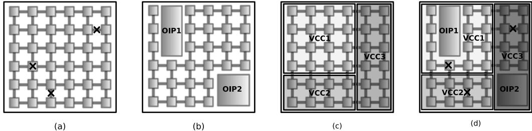
Fig. 1. (a) A faulty  $6 \times 6$  2D-mesh with one node and two links are broken; (b) An irregular mesh with two oversize IP blocks: OIP1 and OIP2; (c) A network with three voltage-frequency islands: VCC1, VCC2 and VCC3, each of them can be powered ON/OFF independently; (d) A hybrid example of all three cases.
