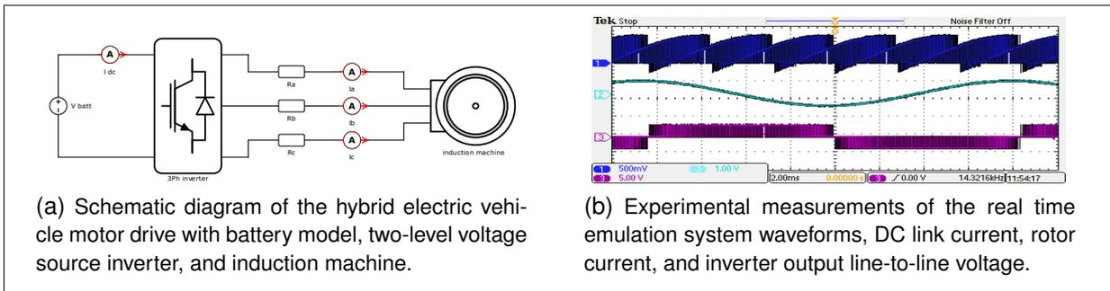
**Figure 6:** Hybrid Electric Vehicle Motor Drive System Application.
