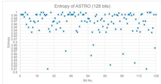
**Figure 8:** The entropies of most bits produced by ASTRO are located between the [0.93, 1] bit window, which is already a good quality. It can be further improved to a [0.997, 1] bit window by the proposed TRNG microarchitecture (cf. Fig. 11).
