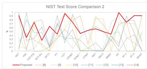
**Figure 13:** If a competitor has more than one design of RNG, the one with the best  $p$ -value is adopted in the figure.
