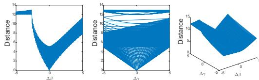
Figure 5: When  $\beta$  (left) or  $\gamma$  (middle) or both of them (right) fluctuate, the attractors will drift away according to the fluctuation magnitude.  $\alpha$  on the other hand is related to the size of the trajectory. Every point with  $\text{distance} \neq 0$  stands for a new chaotic map due to the change made to  $\{\alpha, \beta, \gamma\}$ .
