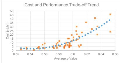
**Figure 10:** The blue dotted trend shows that the quality of the random sequences rises with the energy ( $nJ$ ) consumed per bit.
