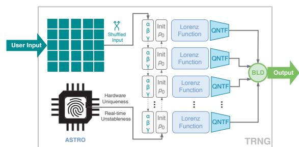
**Figure 3:** The inputs  $(\{\alpha, \beta, \gamma\} \text{ and } p_0)$  of the Lorenz Functions group are run through the SAC network and the ASTRO. Outputs from those units are then passed through the QNTF and BLD modules. The architecture features six tunable parameters for the tuning of the cost-performance trade-off.
