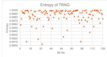
**Figure 11:** The entropy of the TRNG final outputs, which on average is 0.998 bit per output bit. To be comparable with Fig. 8, the TRNG is made to work under 128 bits/cycle throughput.
