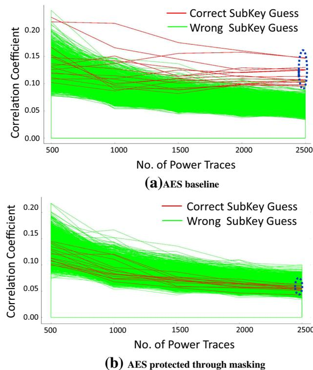
**Fig. 16** Correlation coefficients for AES with or without protection against side-channel attack
