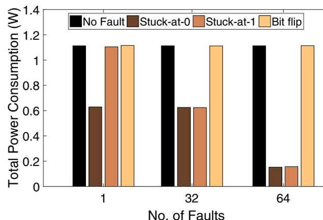
**Fig. 15** Comparison of total power in different fault insertion scenarios
